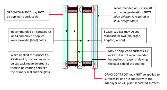
**WARNING**: OPACI-COAT-300® must *NOT* be applied to an interior surface of an IGU if a low-e coating exists on an opposing surface inside the unit. Refer to ICD Technical Bulletin 70-10 OPACI-COAT-300® and Low-E in an IG Unit.
