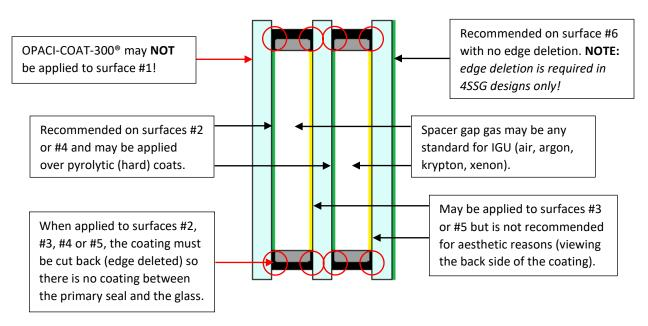
**WARNING**: OPACI-COAT-300® must *NOT* be applied to an interior surface of an IGU if a low-e coating exists on an opposing surface inside the unit. Refer to ICD Technical Bulletin 70-10 OPACI-COAT-300® and Low-E in an IG Unit.
